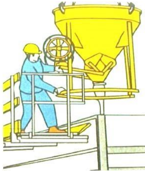
Applying mass concrete
