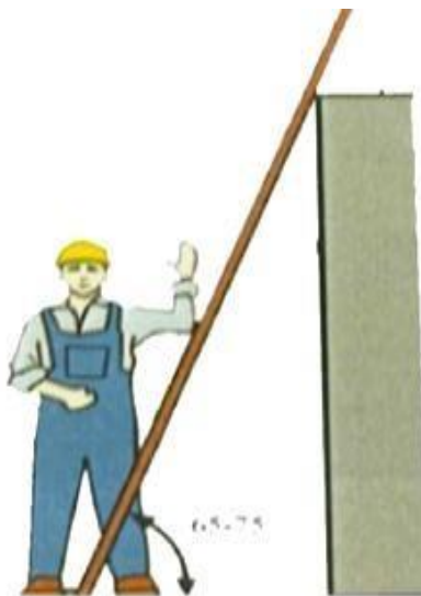
Security exit from deep excavations
